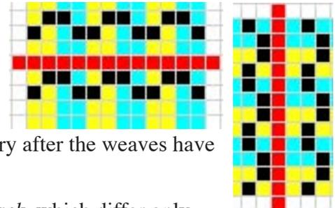
Most Jacquard designs fall into this latter category - so it is always necessary after the weaves have been applied to find and repair the “floaters”.
