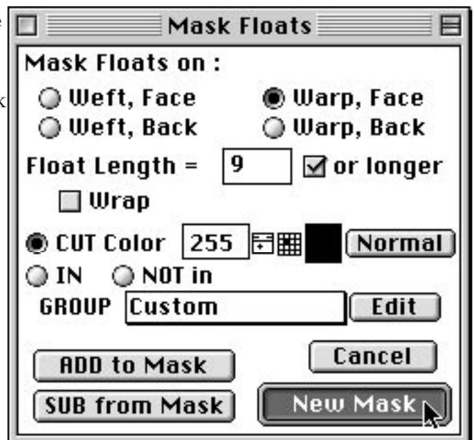
Each warp-face floater shows up as a vertical column of 9 (or more) black pixels. Each floater can be fixed by changing one of those black pixels to a non-black color - which will break it into 2 shorter warp-face floats by forcing the warp to leave the front to cross under a weft.
