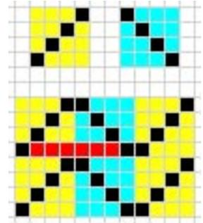
The situation is more complicated when the design features are smaller than the dimensions of the weaves being used - thus preventing each weave from completing full repeats. The Twills in this example are 4x4 while the “features” shown are 2 wide or 2 high. In such cases we can get very long floats indeed!
