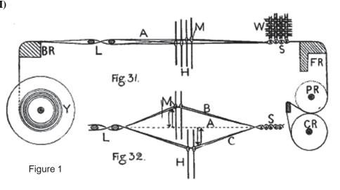
eyes (see Figure 2) for attachment to the mechanism. The shedding mechanism does its work by raising or lowering the heddles, hence the warps.
