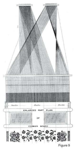
custom made for a particular loom/head and *sley*, also called *sett* or EPI (ends per inch). Changing the harness' sley is not simple - if you move the heddles farther apart the path of the cords changes and their lengths must be re-adjusted.
